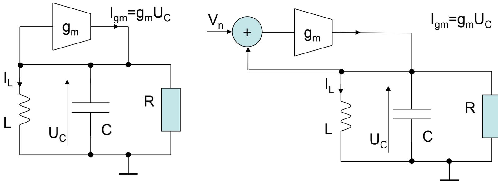
$$K(j\omega) = \frac{g_m}{\frac{1}{R} + \frac{1}{j\omega L} + j\omega C} \quad \frac{dK(j\omega)}{d\omega} = \frac{g_m \left( -\frac{1}{j\omega^2 L} + jC \right)}{\left( \frac{1}{R} + \frac{1}{j\omega L} + j\omega C \right)^2} \bigg|_{\omega = \frac{1}{\sqrt{LC}}} = g_m R^2 j \cdot 2C = 2jRC = \frac{2j}{Q\omega_0}$$
