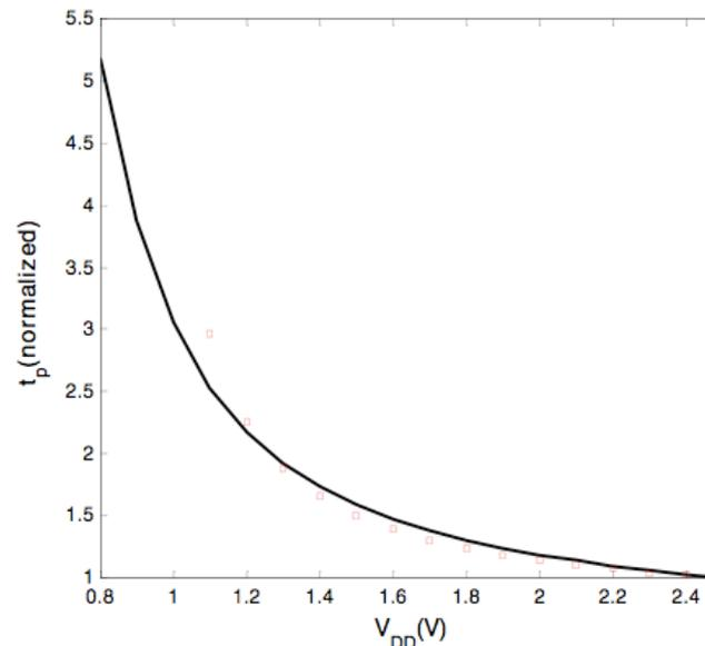
$t_d$  versus  $V_{DD}$ ,
