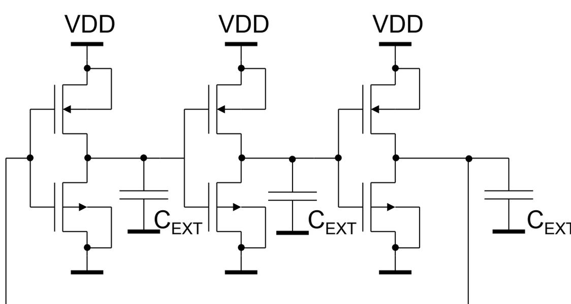
$$t_d \approx \frac{1.6(C_{OUT} + C_{IN} + C_{EXT})}{k'(W/L)V_{DD}}$$
