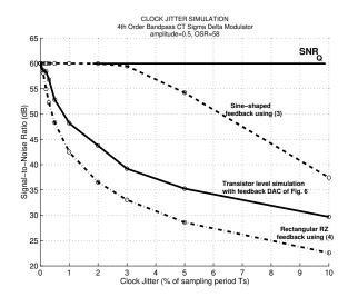
Fig. 8. Comparison of jitter-limited SNR for CT  $\Sigma\Delta$  modulators using, the proposed feedback DAC, a rectangular return-to-zero DAC, and the sine-shaped DAC developed in [2].
