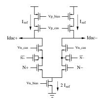
Fig. 6. Proposed sine-shaped feedback DAC, designed in 1.2-V 0.13- $\mu$ m CMOS technology,  $f_s$ =9.768GHz.
